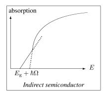
So indirect semiconductors, like Si and Ge, cannot emit any light and are therefore not usable to fabricate lasers. When light is absorbed holds:  $\vec{k}_{\rm h} = -\vec{k}_{\rm e}, \, E_{\rm h}(\vec{k}_{\rm h}) = -E_{\rm e}(\vec{k}_{\rm e}), \, \vec{v}_{\rm h} = \vec{v}_{\rm e}$  and  $m_{\rm h} = -m_{\rm e}^*$  if the conduction band and the valence band have the same structure.
