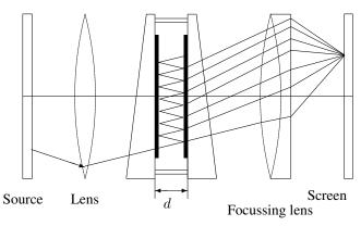
The width of the peaks at half height is given by  $\gamma = 4/\sqrt{F}$ . The finesse  $\mathcal{F}$  is defined as  $\mathcal{F} = \frac{1}{2}\pi\sqrt{F}$ . The maximum resolution is then given by  $\Delta f_{\min} = c/2nd\mathcal{F}$ .
